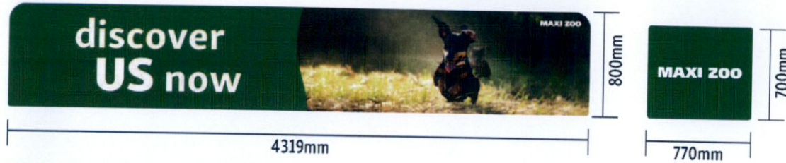
Trolley Bay Graphic Side: 4319x800mm - Matt laminated Print on 3mm Dibond mounted to Stainless Steel frame with pop-rivets
