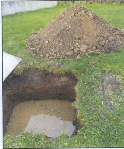
BRE under test
