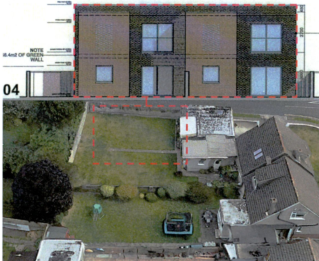
Fig. 44: Overbearing of property to the west's rear garden from 2 no. 6.15m tall houses
