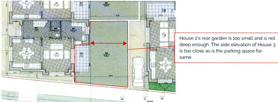
Fig. 26: The compromised siting and design of House 2 (ground level)
