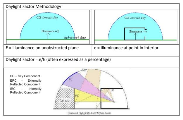
Both illuminances are measured under the same standard sky, a CIE overcast sky. Since the sun is in a particular position for only a short period each day, direct sunlight is excluded. Instead diffuse sunlight is used for average daylight calculations. Diffuse sunlight describes the sunlight that has been scattered by molecules and particles in the atmosphere but has still made it down to surface of the earth.
