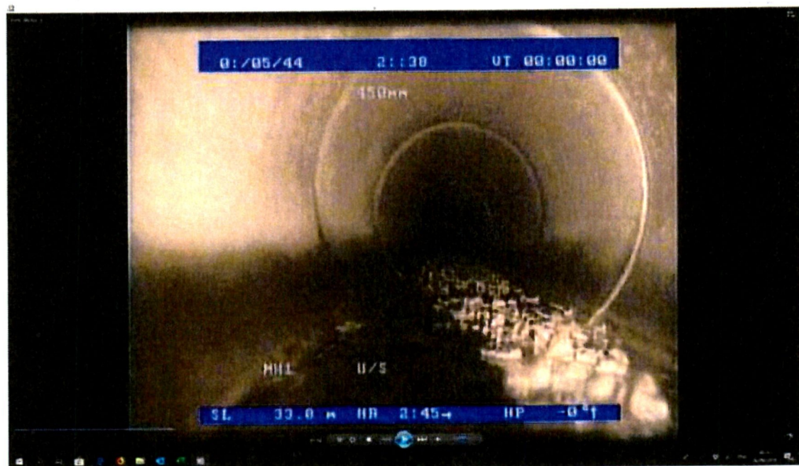
Debris in pipe. No connections
