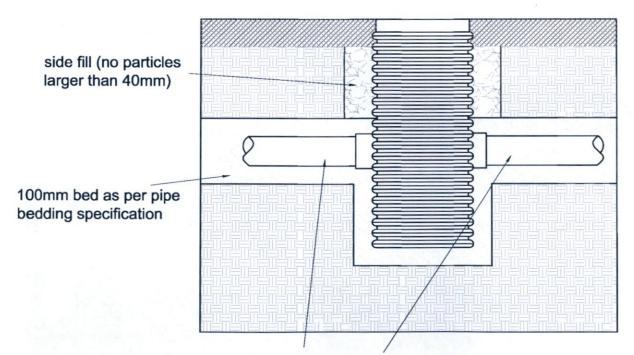
160mm osma drain inlet/outlet or use the appropriate adaptor to connect to the 110mm osma drain
