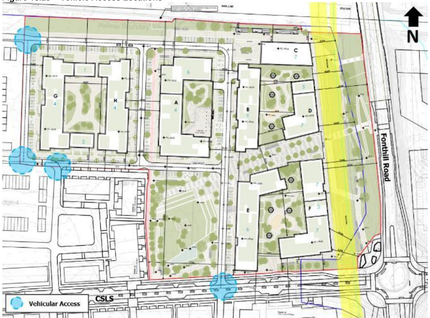
Figure 10.29 – Vehicle Access Locations
