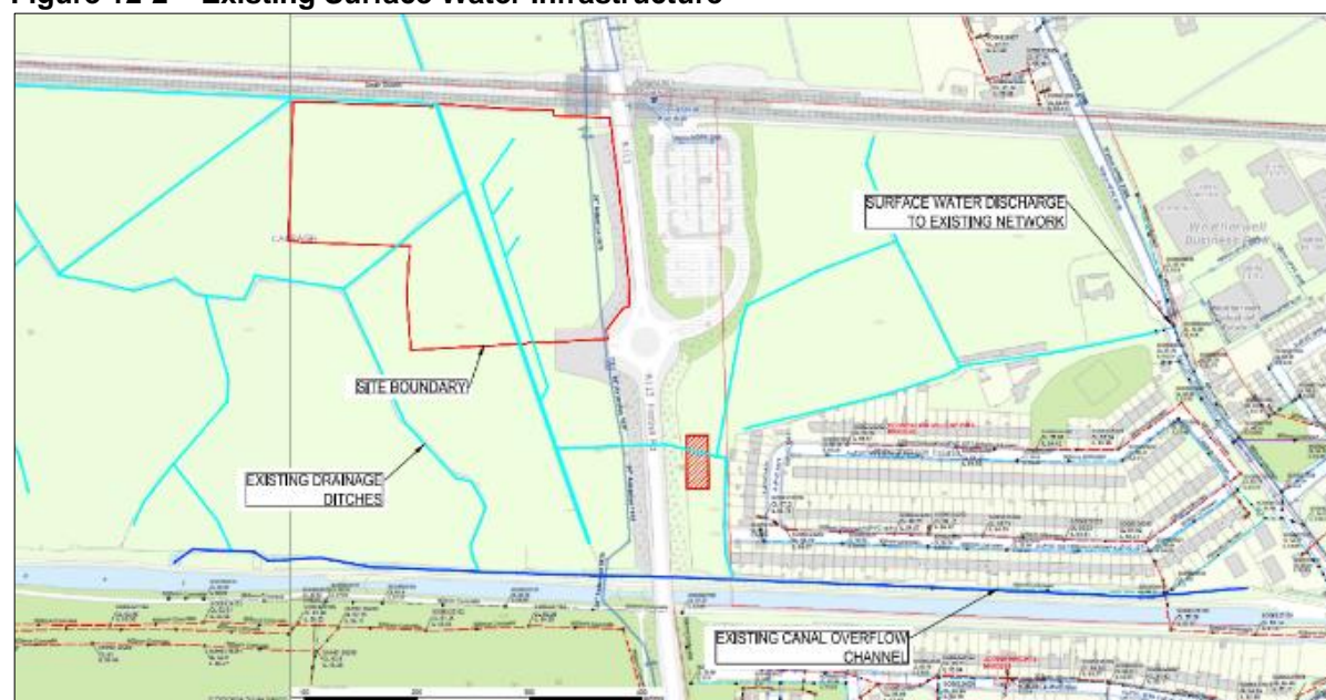
Figure 12-2 – Existing Surface Water Infrastructure
