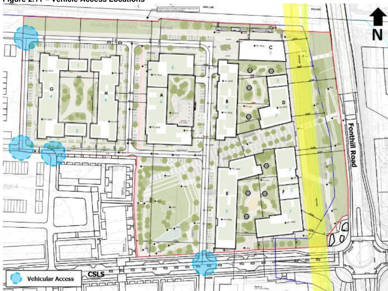
Figure 2.11 – Vehicle Access Locations
