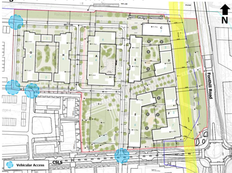
Figure 2.8 – Vehicle Access Locations
