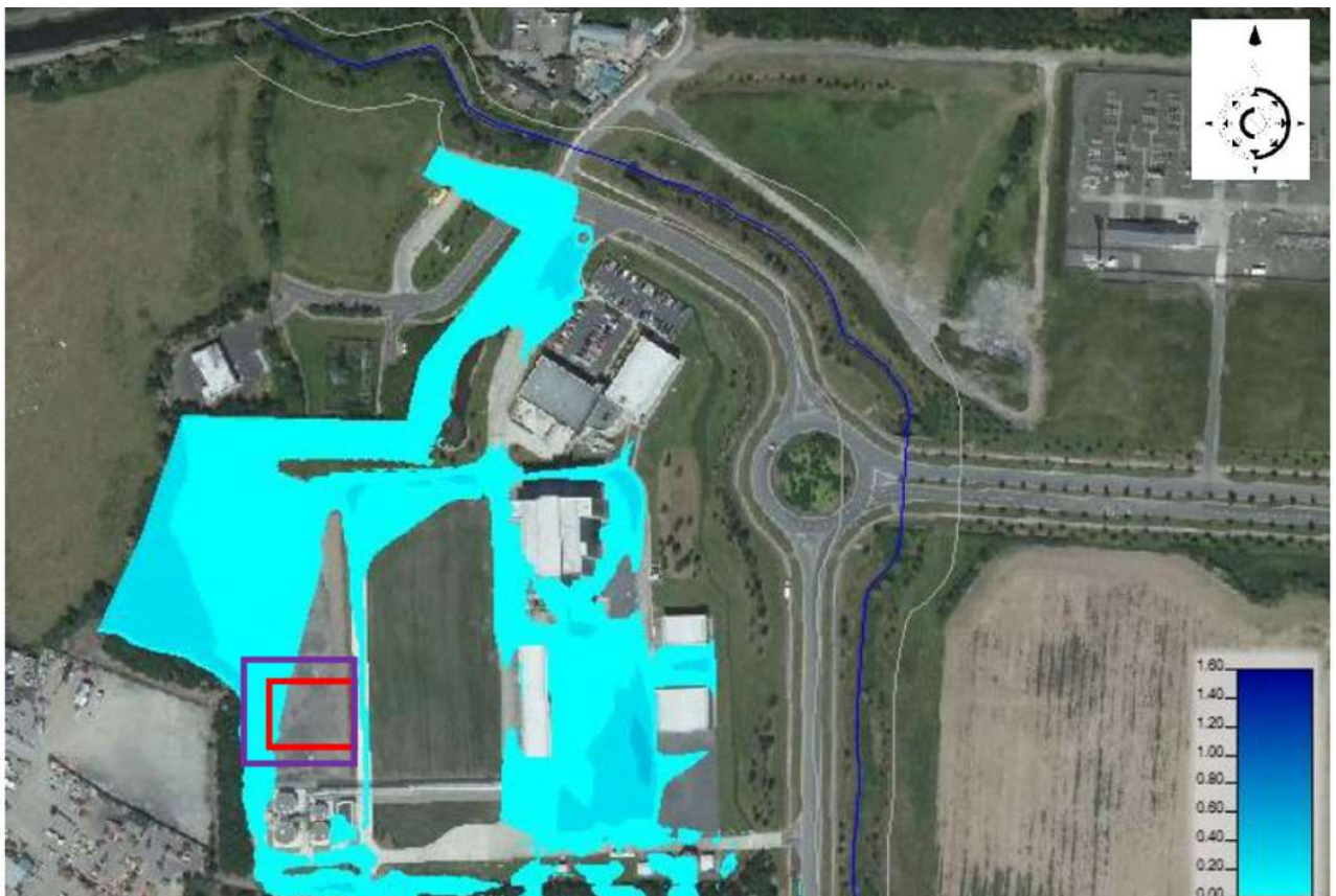
IMAGE - Flood depth on Takeda site for 1% AEP MRFS event (excerpt from FRA stage 3 as submitted with the planning application).
