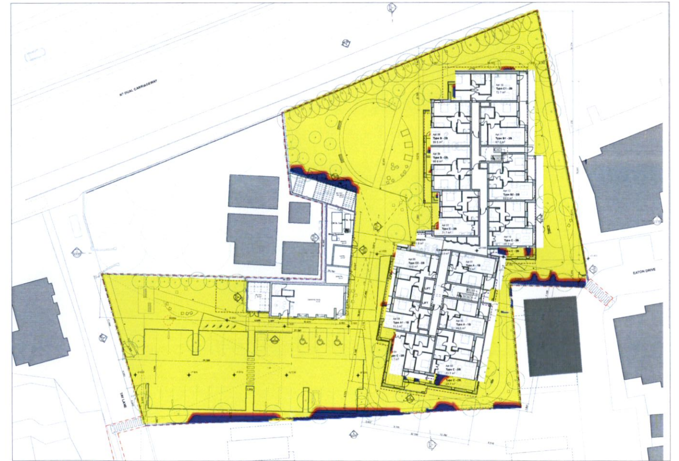
March 21st - More than 2 hours of direct sun to external landscaped amenity areas shown yellow (assuming adjacent site to south east is developed)
