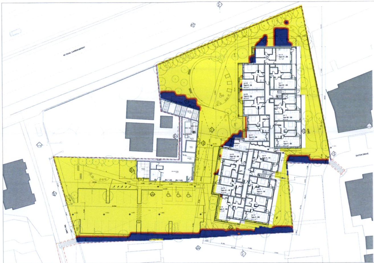
February 1st - More than 2 hours of direct sun to external landscaped amenity areas shown yellow (assuming adjacent site to south east remains undeveloped)
