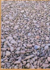
Lower sub-base layer 10-63mm clean crushed stone
