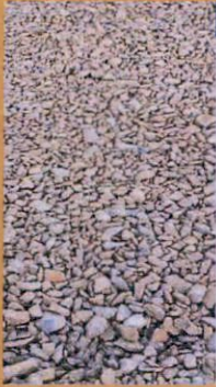
Upper sub-base layer 5-20mm clean crushed stone
