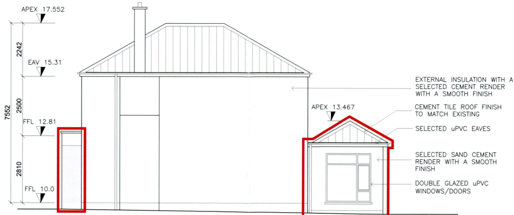
PROPOSED SIDE ELEVATION (SOUTH) SCALE 1 : 100
