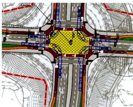
Figure 3-4 Proposed R136 / Link Street Signal Controlled Junction
