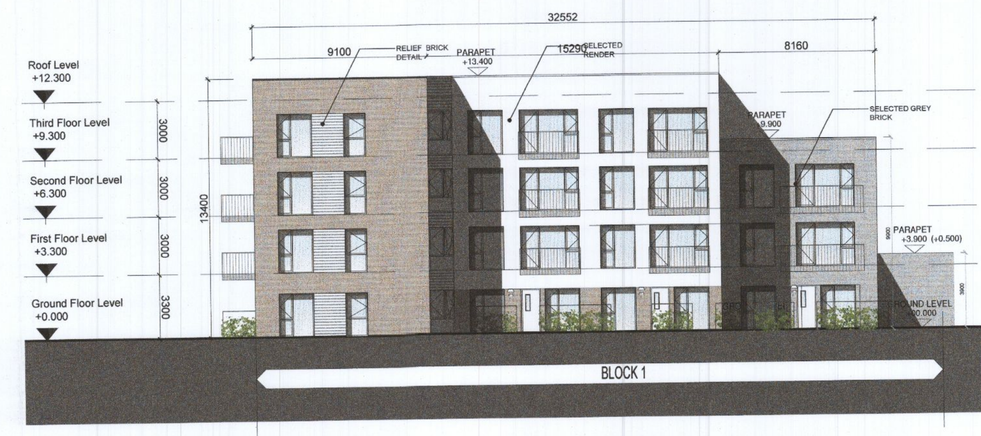
3-BLOCK 1 - SOUTH ELEVATION
