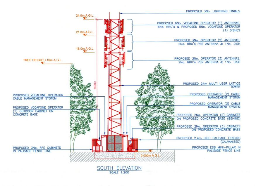
South Elevation Cabin/Cabinet Details PLANNING APPLICATION DRAWING Type: TBC PROPOSED VANTAGE TOWERS SITE AT CHINESE GOSPEL CHURCH, **VANTAGE** Dims: TBC NOT FOR DN415 urvey date 14/06/22 A3 CONSTRUCTION ESKER HOUSE, LUCAN, **TOWERS** Structure Details ved IB - AWAITING PCM Assume all site details are existing unless otherwise specified. DM JPN Co. DUBLIN Type: LATTICE TOWER Height: 24.0m PLANNING APPLICATION DRAWING <sup>)ote</sup> 23/06/22 23/06/22 23/06/22 Drawing No. DN415 / 002 / 06
