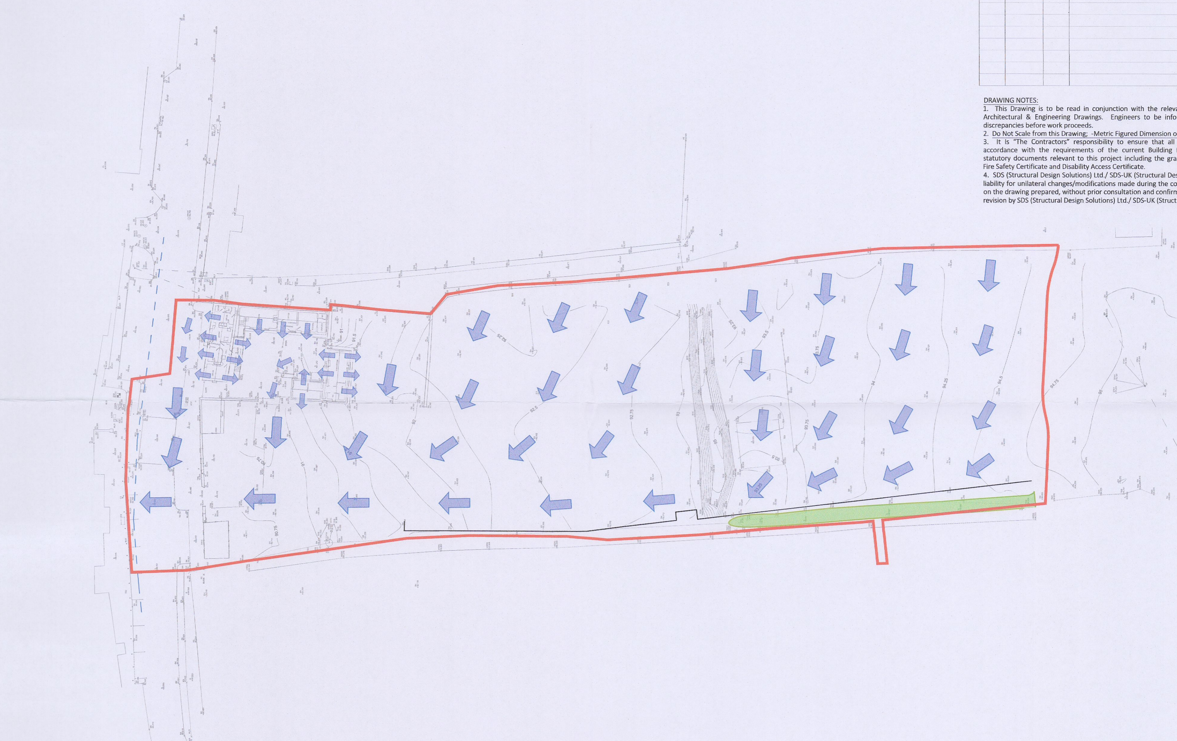
EXISTING SURFACE WATER FLOW PLAN SCALE 1:500
