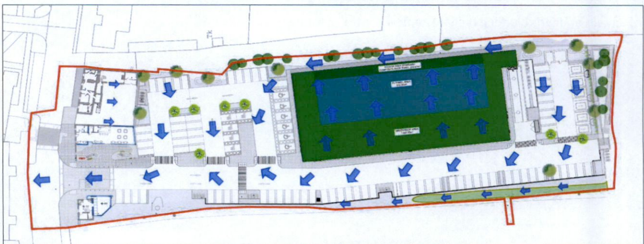
Figure 3.3: Proposed surface water flow plan for site at Newcastle, Dublin
