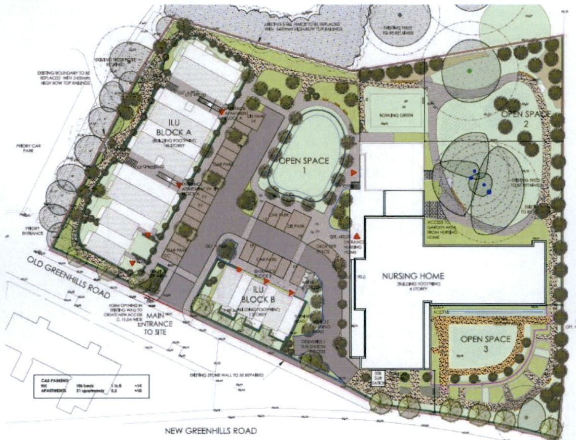
Figure 2.0 Revised site plan showing a much reduced layout with a large quantum of open space.
