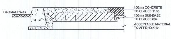
1. FOOTWAY IS SHOWN WITH A IN-SITU CONCRETE KERB TYPE A. ALTERNATIVE KERB TYPES ARE SHOWN RCD/1100/1 AND AT VEHICULAR ACCESS POINTS CONCRETE TO BE REINFORCED WITH A393 MESH REINFORCEMENT TOP AND BOTTOM. ALL CONCRETE EDGES AND JOINTS SHALL BE BULLNOZED WITH A TROWEL.
