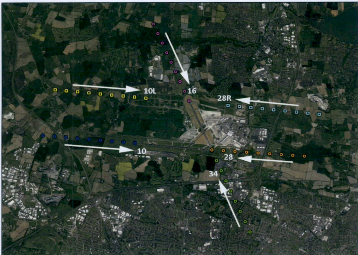
Figure 4: Aerial view (Google Earth Pro) showing 2 mile approach lines to runways at Dublin Airport (at ¼ mile intervals) as assessed by SGHAT. Includes the newly opened northern runway (10L and 28R).
