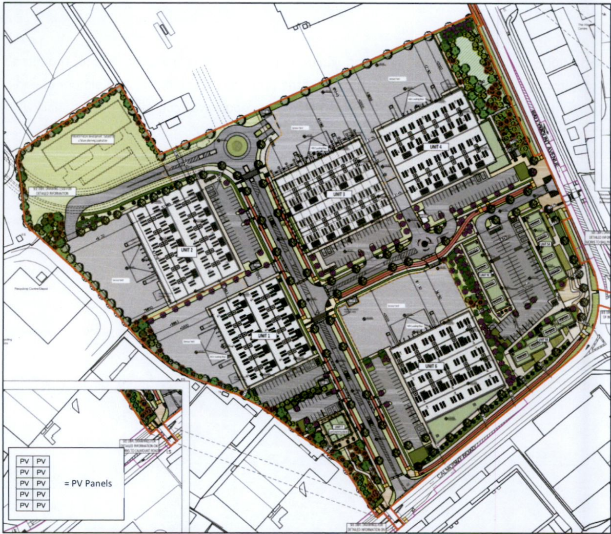
Figure 2: Extract from drawing '18-42-CFI-171-Proposed Site Plan' indicating the location of the proposed PV panels.
