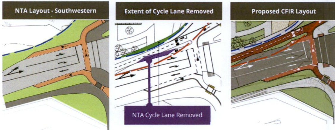
Figure 4.7: Amendment to NTA CBC Cycle Lane on Calmount Rd (Extract of DBFL drawing 210175-DBFL-TR-SP-DR-C-1121)
