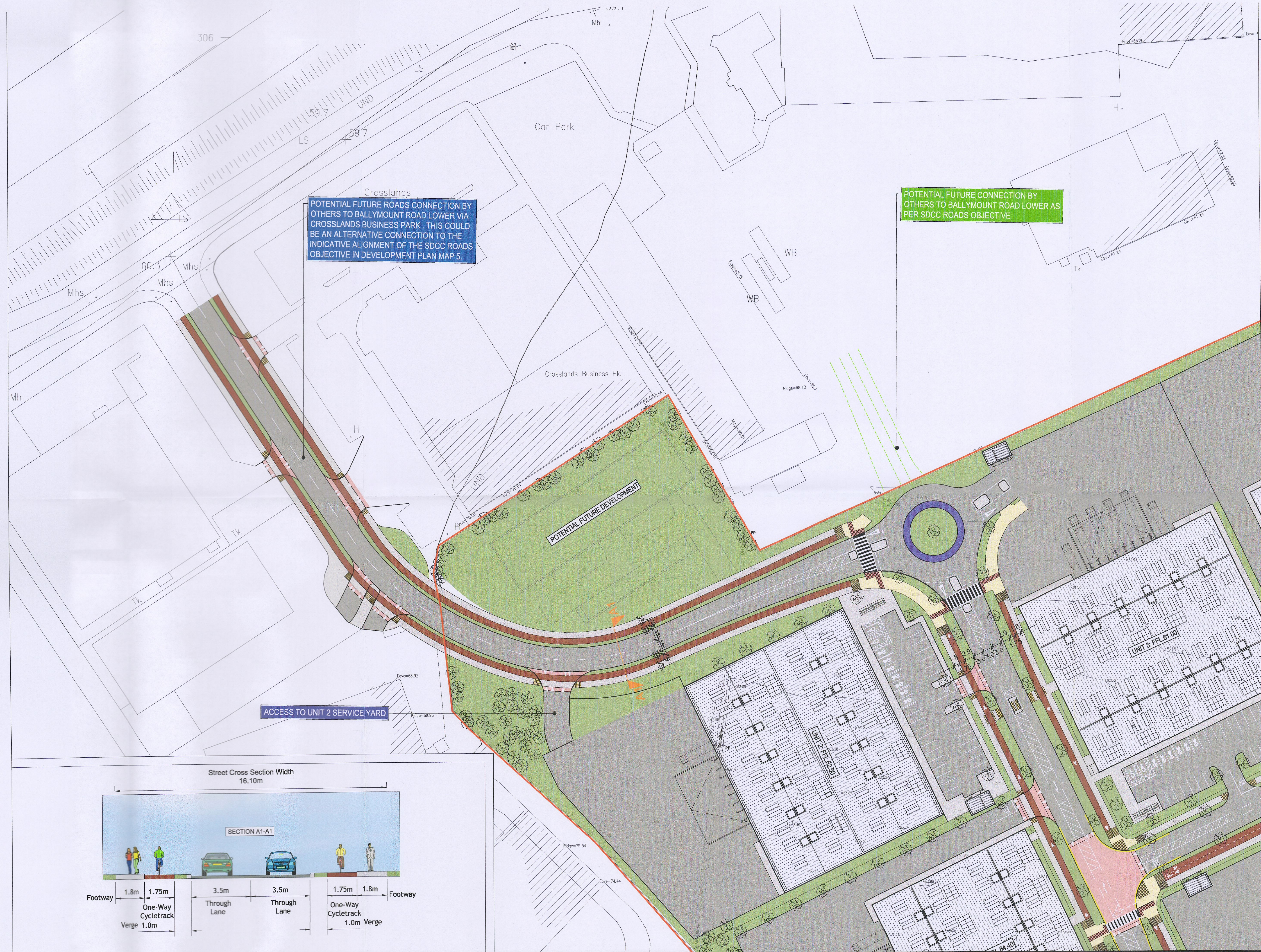
V1 - CROSS SECTION A1-A1 PROPOSED CROSS THROUGH FUTURE BALLYMOUNT LOWER CONNECTION
