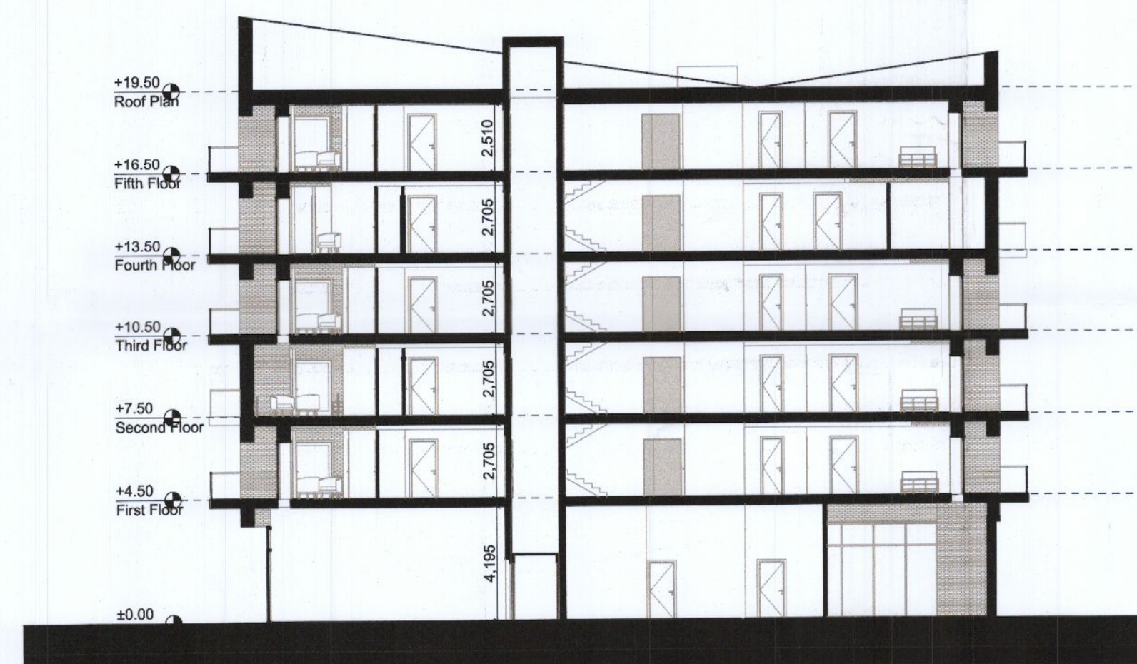
4 Typical Cross Section
