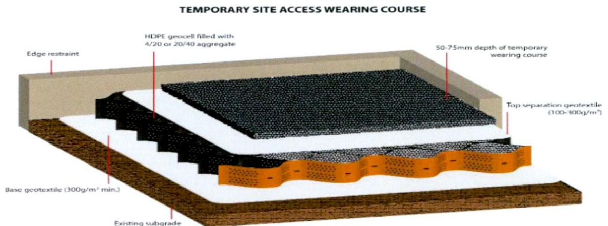
FIG 3 – Top separation geotextile to stop mud from entering infill
