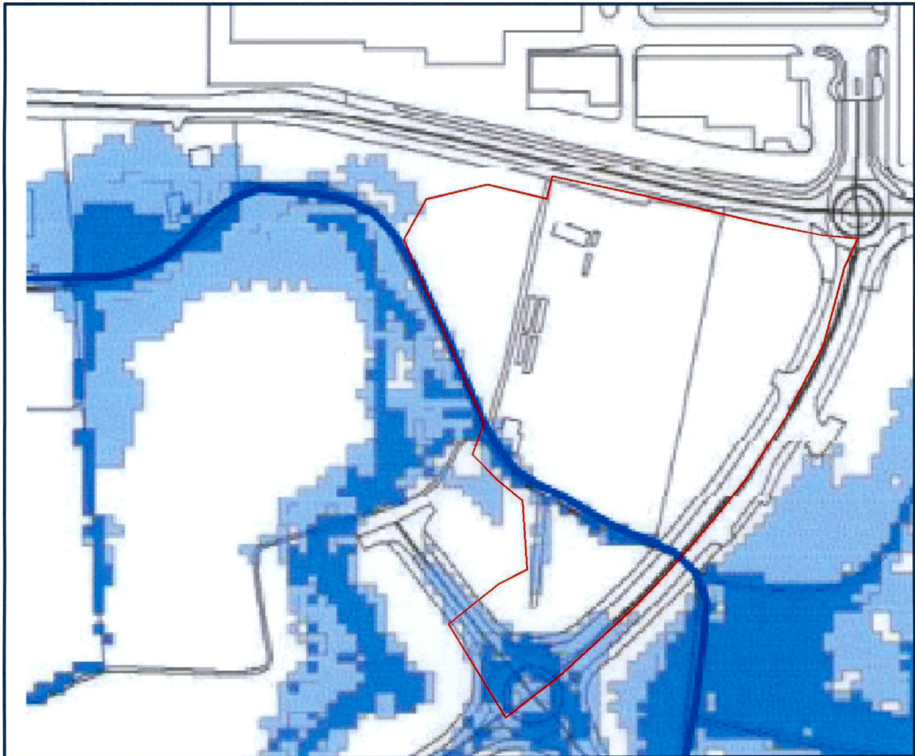
Figure 5-1 Extract from SFRA showing fluvial flood risk at the Site
