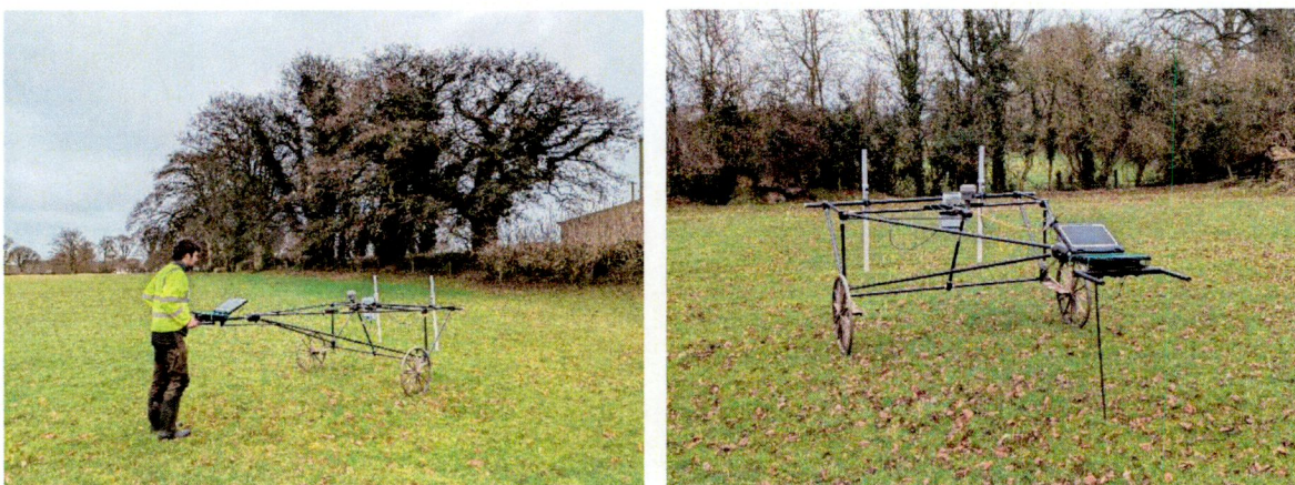
Bartington Grad 601-2 mounted on Bartington Cart system
