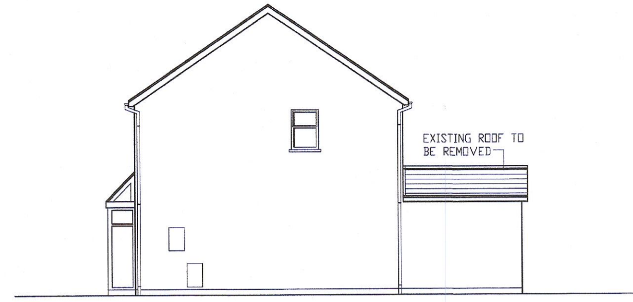
EXISTING GABLE ELEVATION SCALE 1:100
