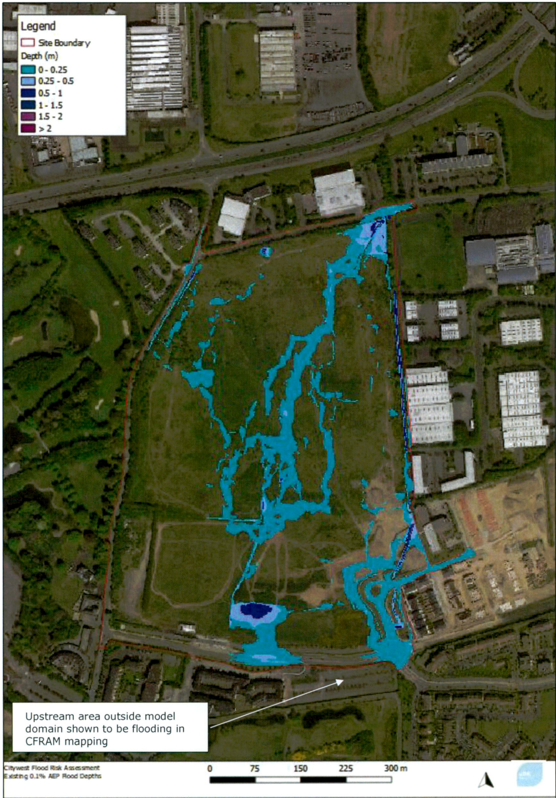
Figure 4-4: Existing 0.1% AEP flood risk
