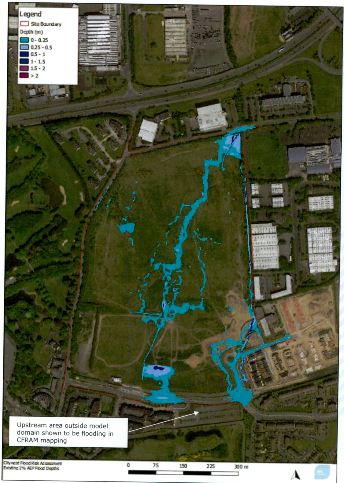
Figure 4-3: Existing 1% AEP flood risk
