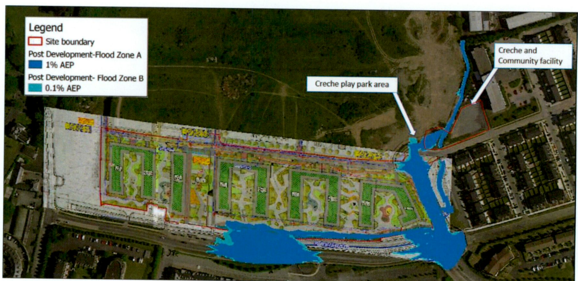
Figure 2-2: Post development 1% AEP and 0.1% AEP MRFS Peak Flood levels (indicative Subject site red line) [Source CityWest Flood Risk Assessment by JBA consulting 2019]
