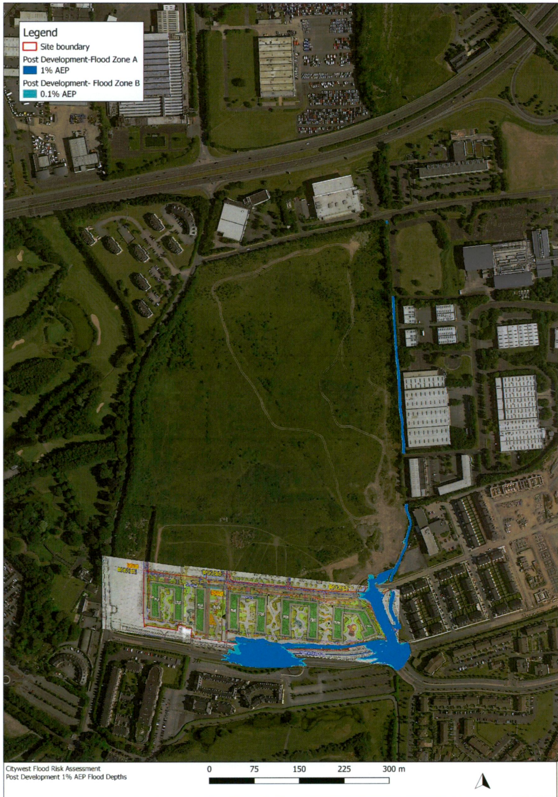
Figure 4-5: Post Development- 1% AEP & 0.1% AEP Flood Extent
