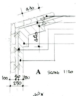
100 new selected stone structure. 50 cavity. stainless steel masonary ties. 100 concrete block with clean
