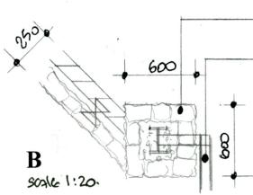
600x600 selected stone pier to match new stone front boundary walls. new selected aluminium entrance gates fixed to steel frame in insith concrete by specialist.
