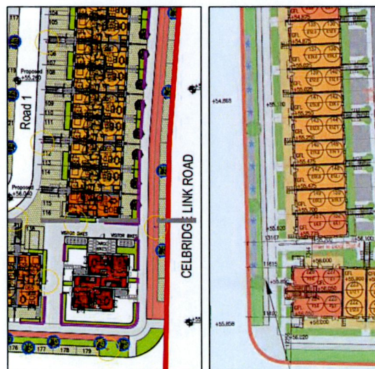
Figures 5.4 and 5.5: Proposed street tree locations at Celbridge Link Road, between car parking spaces – Phase 3 (left) and Phase 2 (right, Reg. Ref. SDZ21A/0014) just north of the Celbridge Link Road and Adamstown Way junction.
