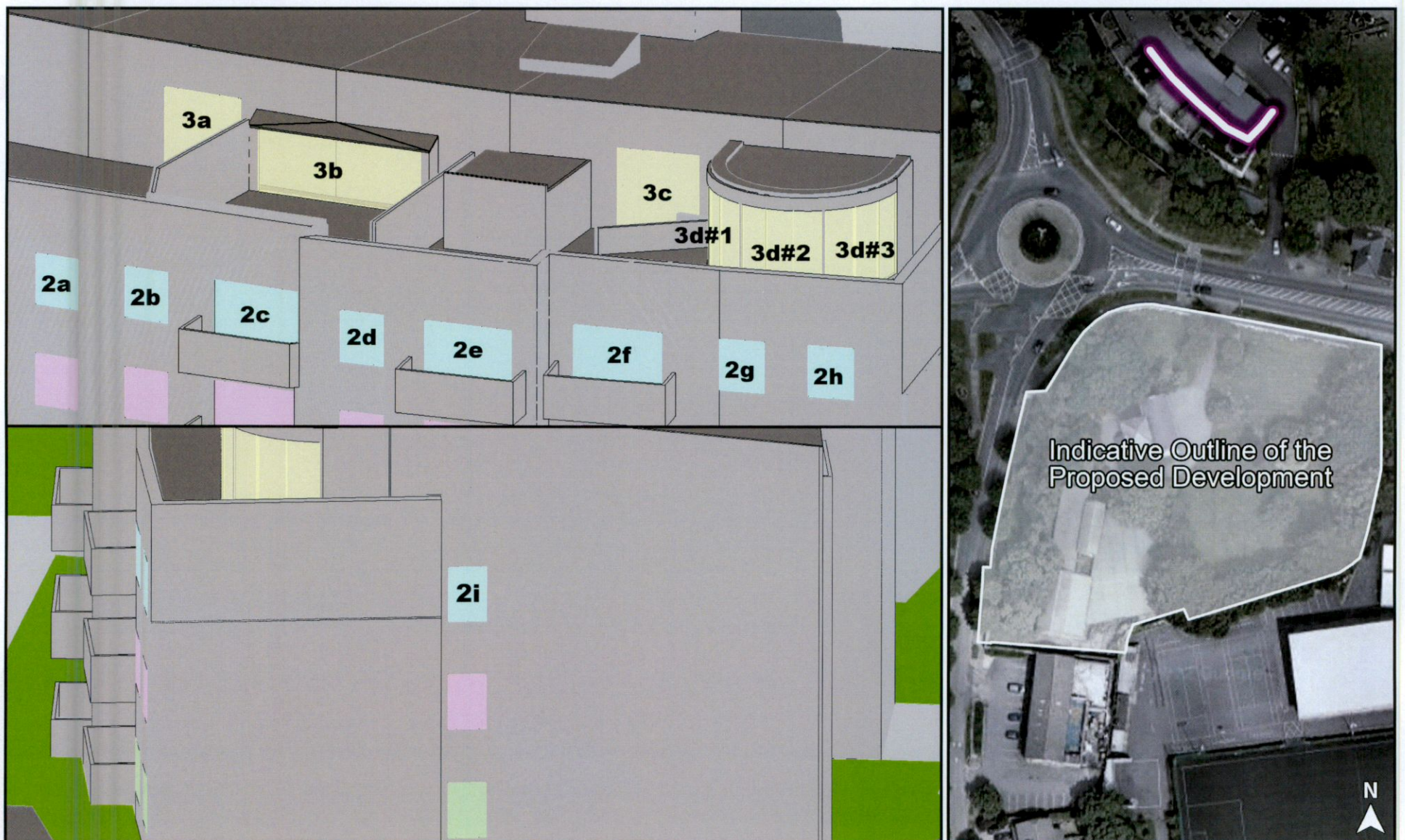
Figure A.16: Highlighted areas indicate the position of assessed windows (L), Aerial view of assessed location (R)
