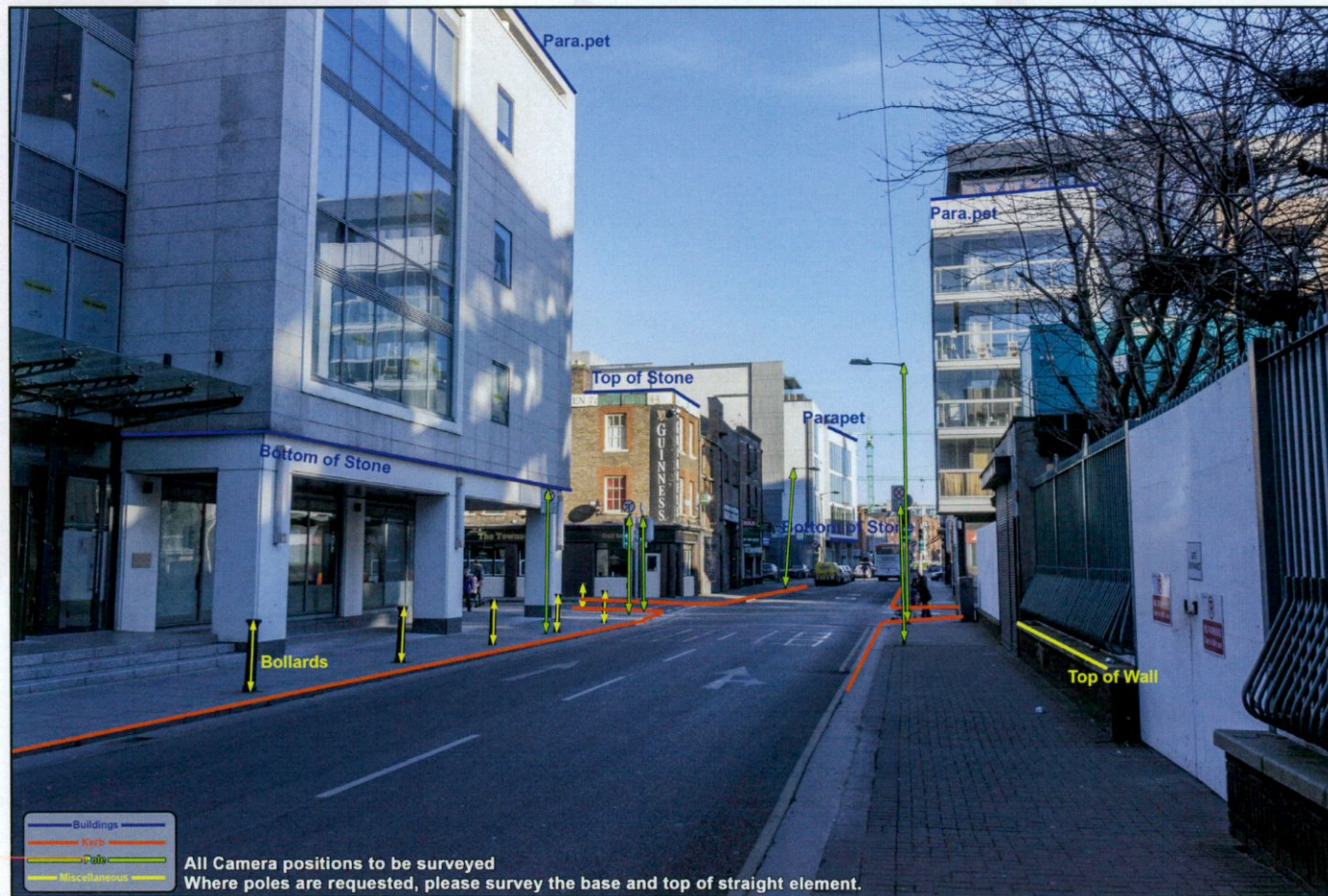
Fig.7: Fixed reference points marked for surveyour.
