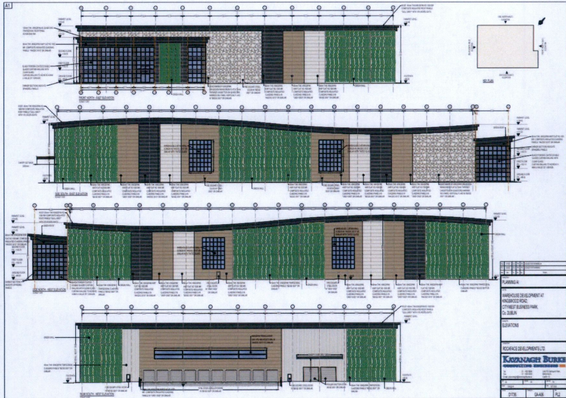
Figure 2: Elevations and proposed green walls
