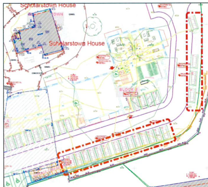
Figure 19: No provision for footways adjacent to parking areas
