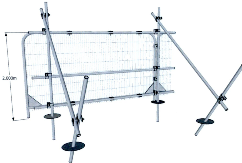
Figure 1. Protective fence specification
