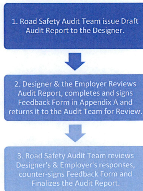
Figure 4.1 – Road Safety Audit Sign-Off and Completion Process
