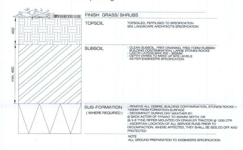
Detail D 01 Drawing LD-04-PP Topsoil depths and Bark Mulch specification to planted areas Scale @ 1:20
