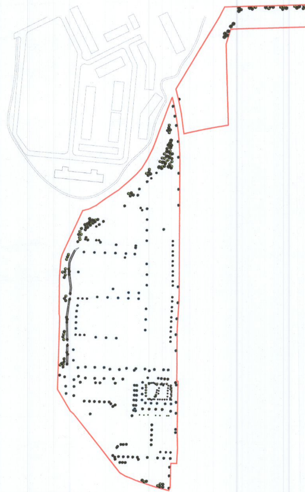
Proposed new street trees 161 no. Proposed new open space trees 202 no. Proposed bio retention tree pits 108 no. Proposed swales, total length 150 linear mtrs
