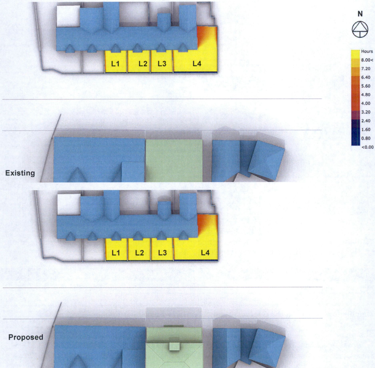
Figure 5: Existing & Proposed Radiation map of amenity areas, showing available sunlight on 21st March. The scale represents the percentage of daylight received from 0 - 8 hrs.
