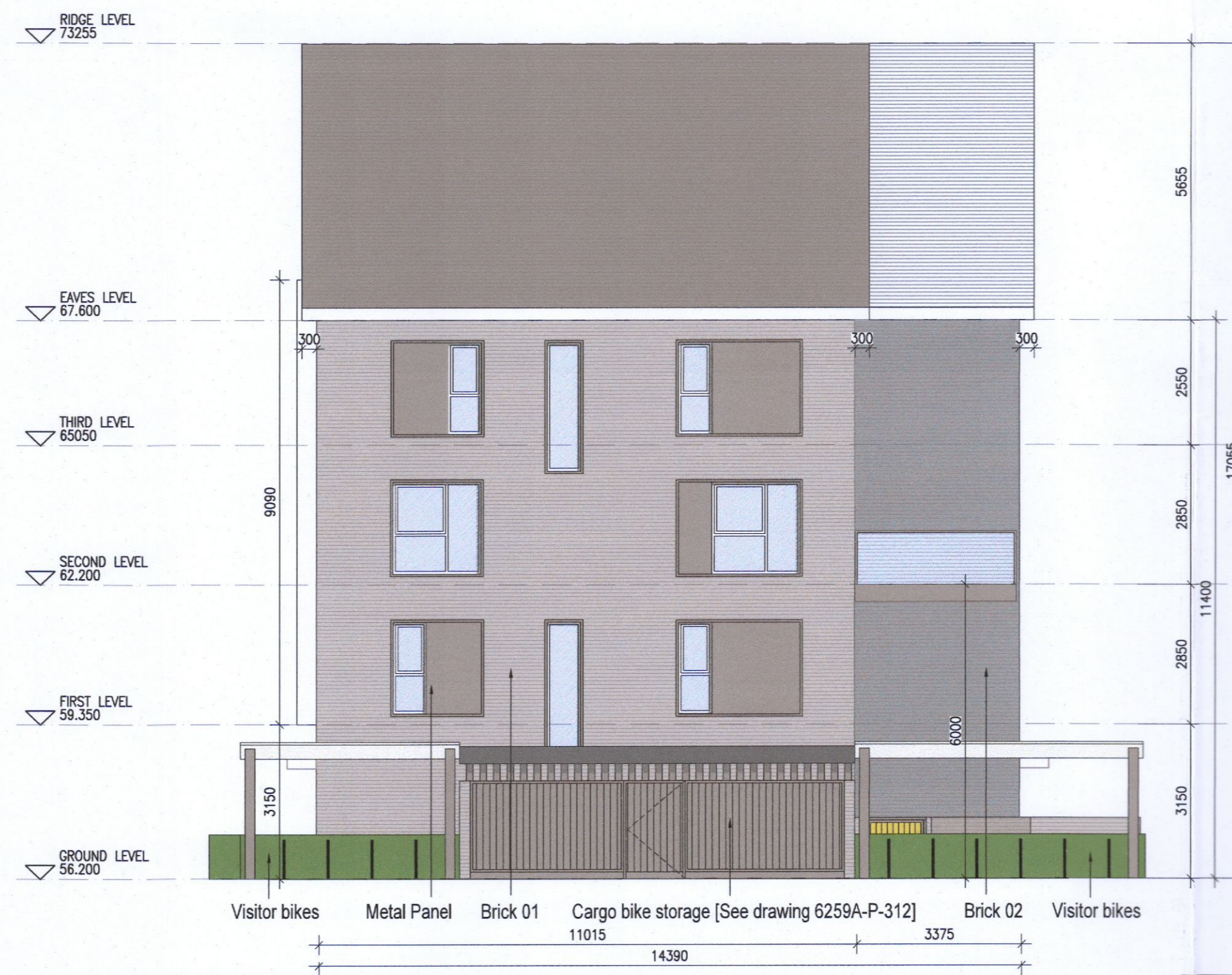
04 Side (North) Elevation H1/H2 1:100@A1
