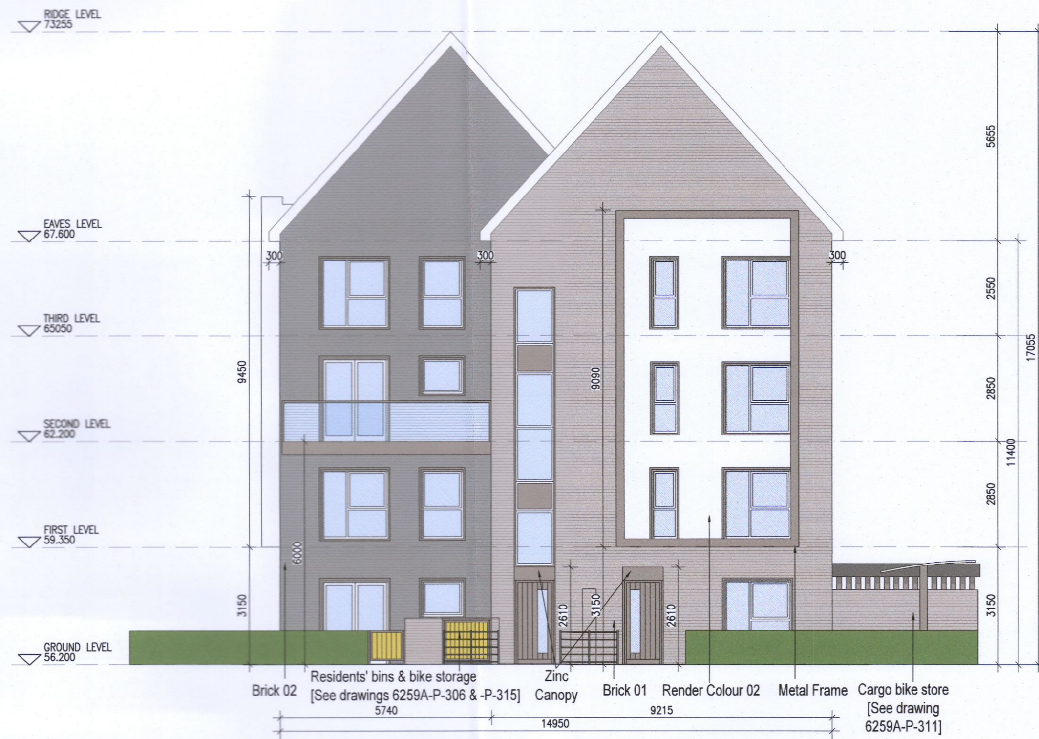
01 Front (East) Elevation H1/H2 1:100@A1
