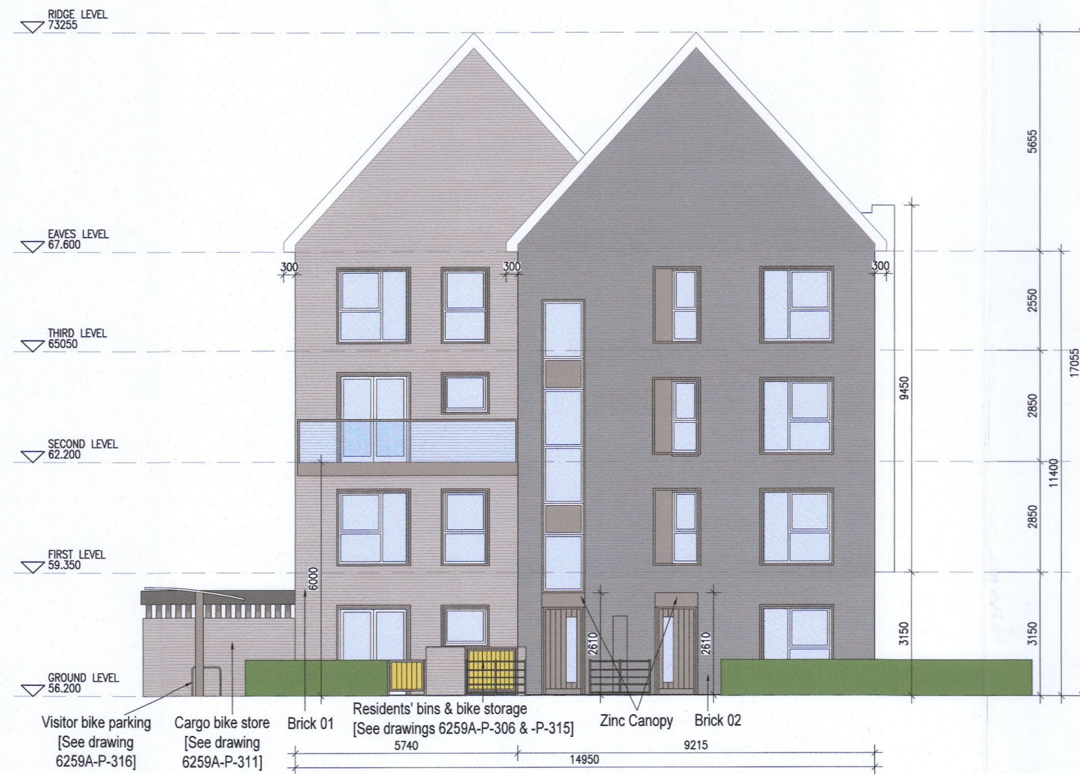
02 Rear (West) Elevation H1/H2 1:100@A1
