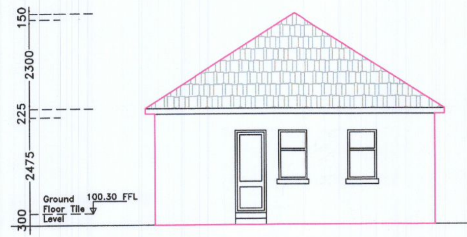
SIDE ELEVATION (WEST) (PROPOSED) SCALE 1:100
