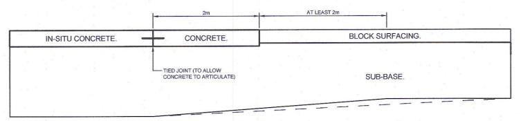
IN-SITU CONCRETE TO BLOCK SURFACING (NO ROAD BASE)
