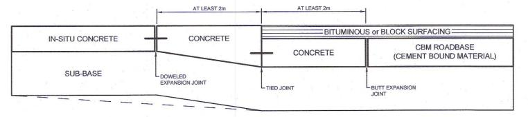
IN-SITU CONCRETE TO BITUMINOUS OR BLOCK SURFACING (WITH ROAD BASE)
