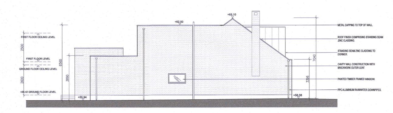
PROPOSED SIDE/EAST ELEVATION SCALE: 1:100
