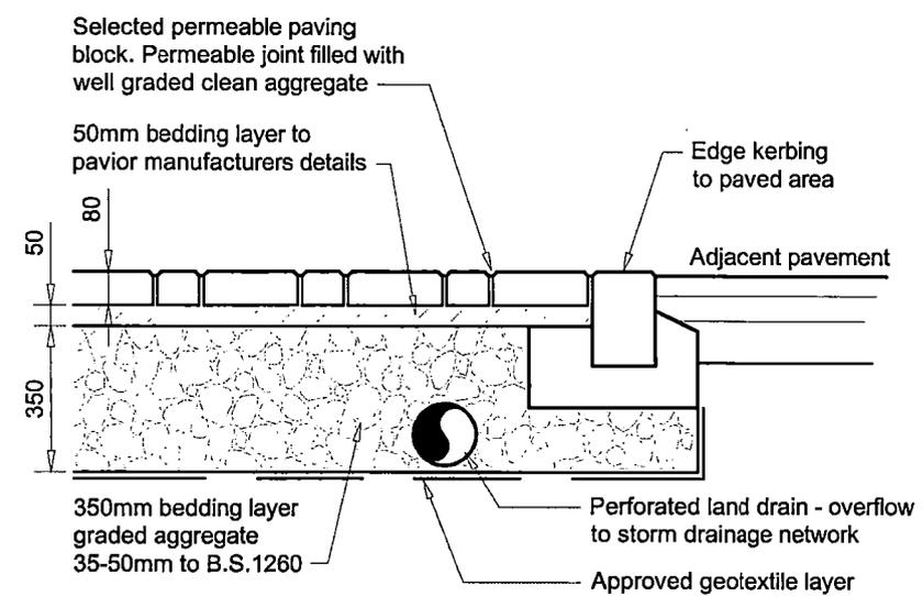
**PERMEABLE PAVING DETAIL**
