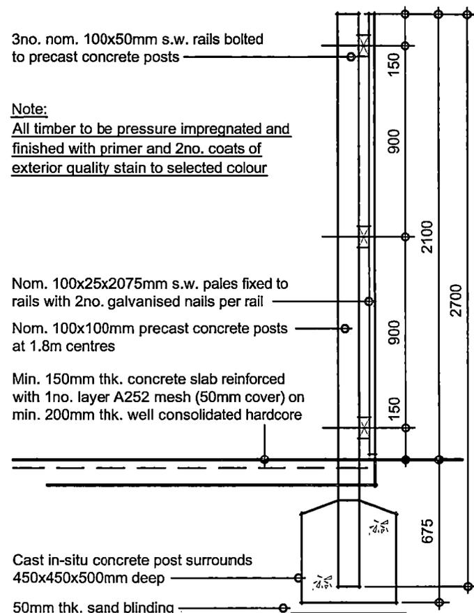
3no. nom. 100x50mm s.w. rails bolted to precast concrete posts
