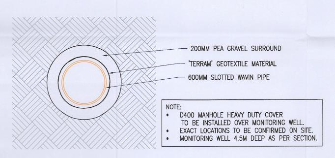
MONITORING WELL DETAIL SCALE 1:25
