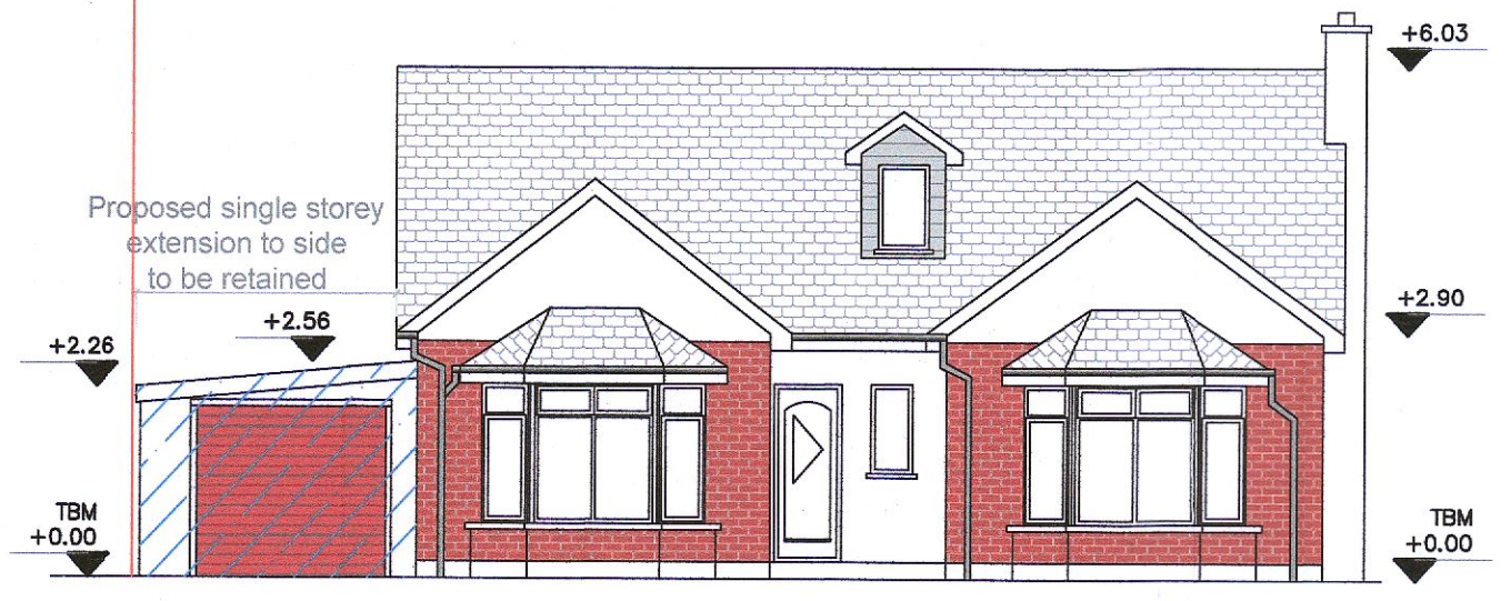
Proposed Front Elevation Scale 1:100
