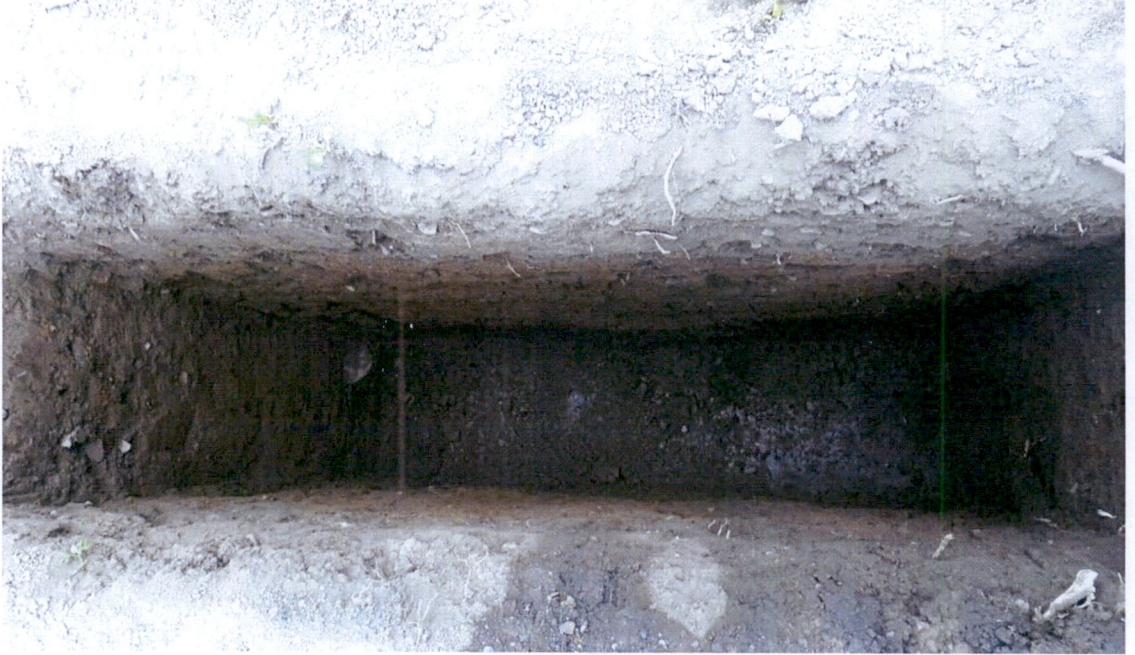
Test Pit before water added – Depth 0.8m
