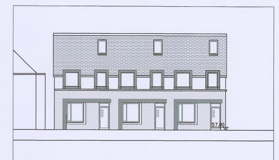
PROPOSED NORTH (FRONT) ELEVATION OF NEW HOUSES (1:200)
