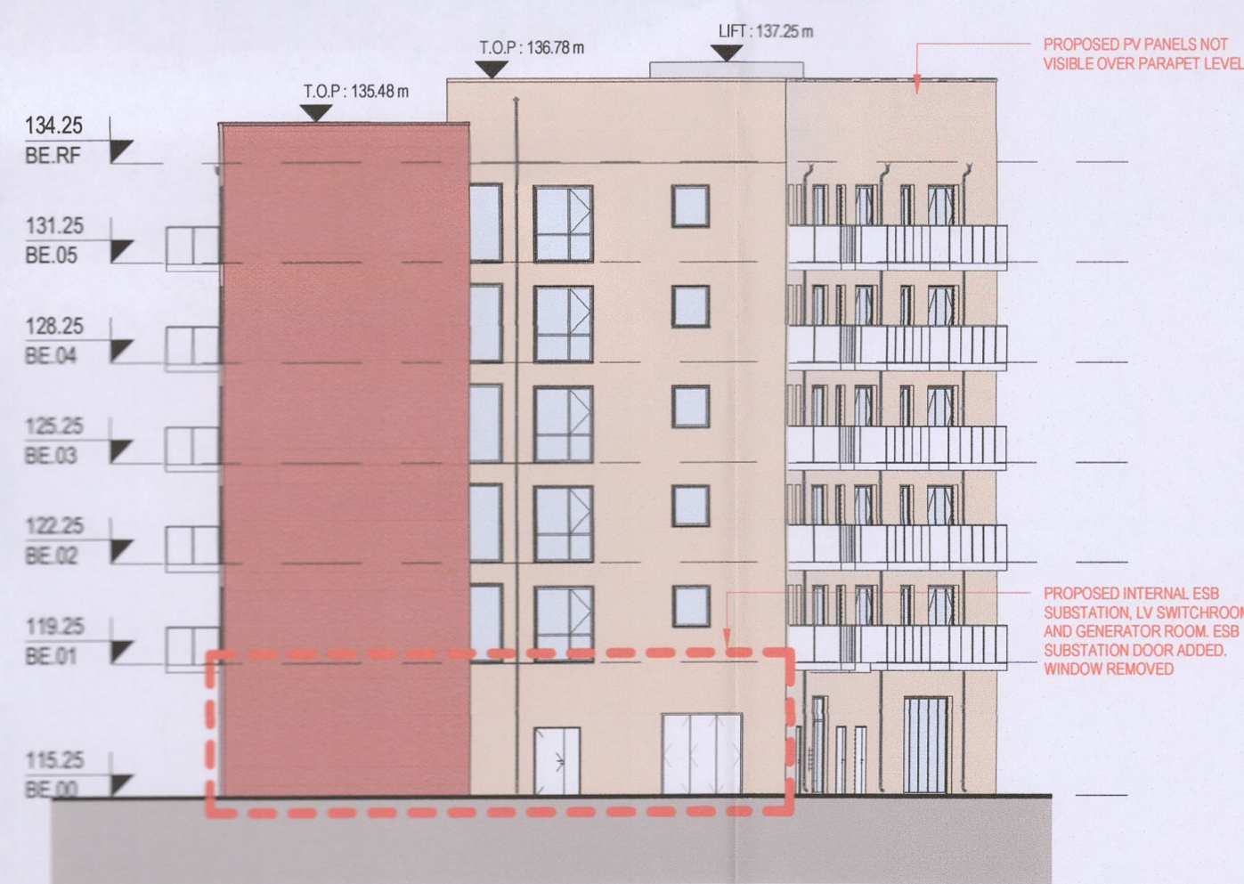
3 PROPOSED - BLOCK E - SOUTH ELEVATION Scale: 1 : 200
