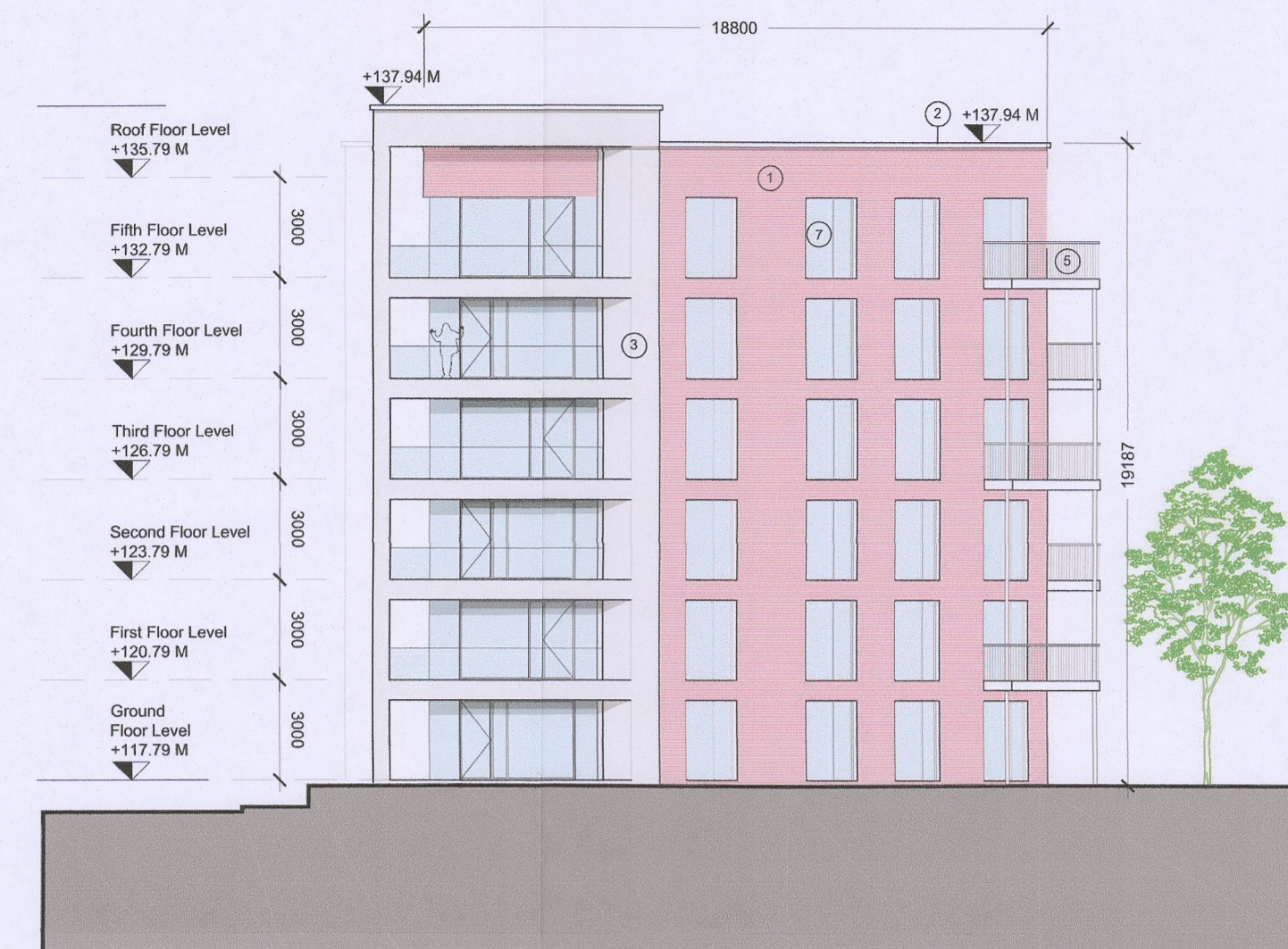
2 PERMITTED - BLOCK A - WEST ELEVATION - PLANNING REF ABP-305556-19 Scale: 1 : 200
